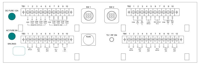
For 2 coax switches and 2 antennas, IBOC or analog. Safe switching from a single momentary local or remote command. Logic for a third transmitter is programmed.
