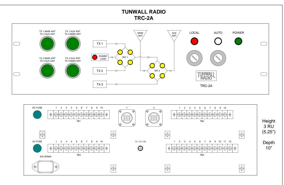
For 2 coax switches and 2 antennas, IBOC or analog. Safe switching from a single momentary local or remote command. Logic for a third transmitter is programmed. Automatic plate on and off for all 3 transmitters.
